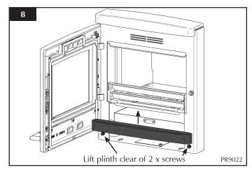
8.3 If the plinth is too loose it can be adjusted via the 2 x side screws and half lock nuts behind it. The plinth is designed to sit tight but still be removable.
