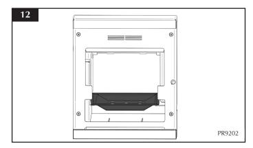
Fit the plug supplied into the hole where the riddling mechanism is normally located and secure with bolt and clamp (also supplied, see Diagram 13).
