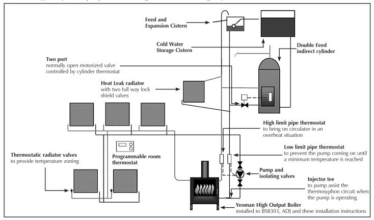
See below a typical layout of a fully pumped central heating and hot water circuit:
