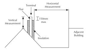
The datum for vertical measurement is the point of discharge of the flue from either the point of discharge of the flue or 150mm above insulation, whichever is the lower.
