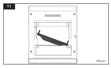
Place tray flat on the fixings on the firebed (see Diagram 12).
