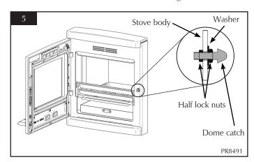
7.3 Ensure the dome catch is in an upright position with the flat sides parallel with the side of the stove (see Diagram 6).
