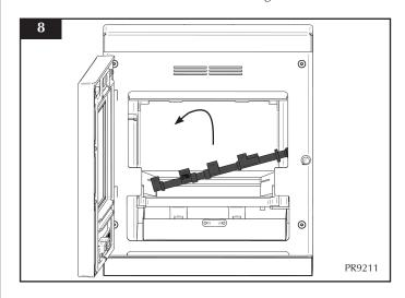
6.7 Lift the multi-fuel frame and rotate to remove from the firebox.
