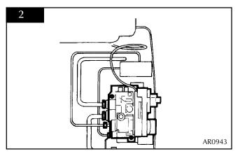
2.3 • Loosen main injector nut on airbox and disconnect from injector, see diagram 3, A.
