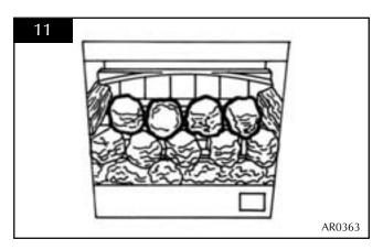
5.7 • Put the remaining three coals behind the last row to touch the back panel, see diagram 12
