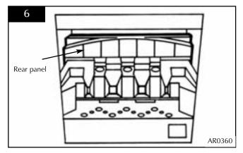
6.3 • Put the front coal between the heat shield and flame baffle
