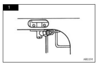
Disconnect thermocouple from gas valve. See diagram 2.Remove ignition lead from electrode. (Cut cable tie to ignition lead if required).
