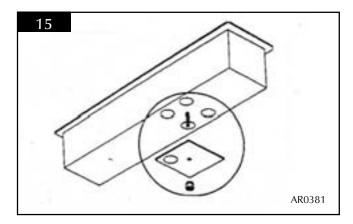
10.2 • Remove the plate and replace with the correct size
