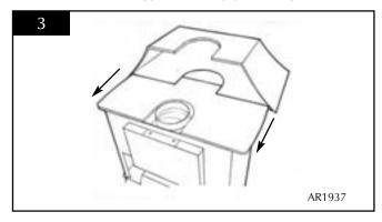
• Make sure the stove top fits into the guide along the bottom of the canopy, Diagram 4
