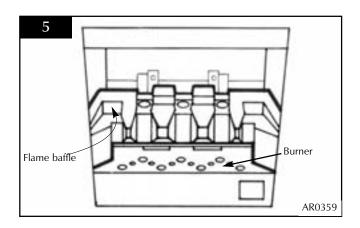
6.2 • Put the rear panel back to the spacer brackets• Slide down so that it locates on the ledge of the flame baffle, Diagram 6
