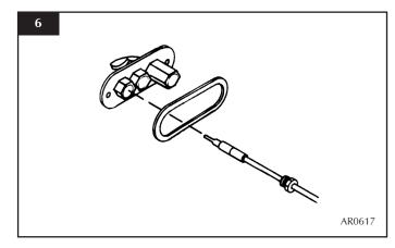
3.15 Undo the thermocouple at the gas valve end (see Diagram 7, A).
