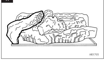
6.7 Put the groove underneath Log F onto Log C (see Diagram 12) so that Log F is parallel to the side of the firebox (see Diagram 13).
