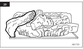
4.11 Put the groove underneath Log F onto Log C (see Diagram 21) so that Log F is parallel to the side of the firebox (see Diagram 22).
