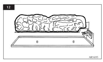
4.6 Place Log C onto the two studs on the burner skin (see Diagram 13) with charred effect of the log facing forward (see Diagram 14).
