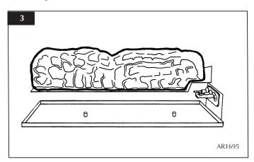
6.2 Place Log C onto the two studs on the burner skin (see Diagram 4) with charred effect of the log facing forward (see Diagram 5).
