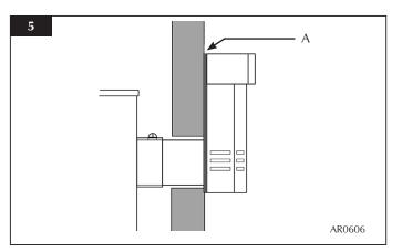
3.26 Feed the flue through the wall, making sure it runs smoothly.
