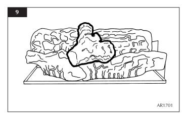
6.6 Position Log B so that the underneath rests in the groove of Log C (see Diagram 10) and the end is in the corner of the burner (see Diagram 11).
