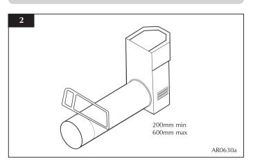
Terminal dimensions: 395 x 200 x 200 mm (H x W x D) Guard supplied Cut to length as required on site (see Diagram 2).
