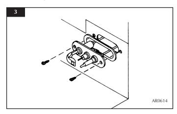
3.6 Carefully draw the pilot assembly away from the firebox. You now have access to the nuts and ignition lead.
