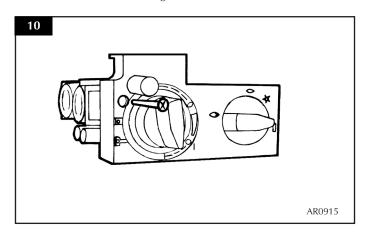
6.4 To release the right hand side of the control cover insert the narrow blade screwdriver into the slot shown in Diagram 11. Lever it gently and pull from the right hand side at the same time. The cover will now come off. There is a small cylindrical metal spacer inside the cover, this must be kept and replaced on the fixing screw during re-assembly.
