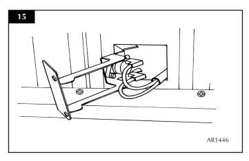
9.3 Refit the new sensor ensuring that the plastic spacers are located between the bracket and the sensor. Refit the leads (see Diagram 16).
