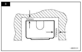
The above dimensions provide adequate clearance to combustible materials. It may be necessary to add additional clearance so that the controls can be reached and spillage tests performed when necessary.
