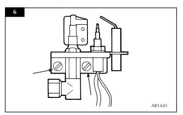
3.4 Reassemble in reverse order, do not overtighten. NOTE: SPECIAL CARE SHOULD BE TAKEN WHEN REPLACING THE THERMOCOUPLE TO THE BACK OF THE GAS VALVE TO ENSURE THAT THE SENSOR WIRES FOR THE GAZCO FLUE SURE SYSTEM ARE NOT DISCONNECTED.
