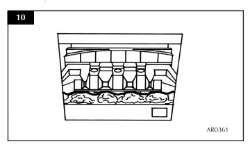
4.10 Place five of the loose round coals on the front coal so that they lean against the flame baffle, in between the fingers. Place the two rectangular coals against the reflector panels, one either side, behind the front row of loose coals (see Diagram 11).
