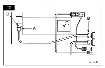
8.3 Reassemble in reverse order. The injector must **NOT** be tightened into the burner but be allowed to float to enable it to line up with the pipe. Turn on the gas supply and check for leaks.
