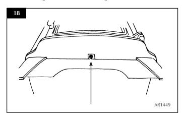
10.2 Undo the M5 nyloc nut from the bottom of the burner unit and remove the aeration plate (see Diagram 19).
