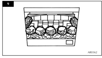
6.6 Place four of the loose round coals behind the first row so that they sit on the fingers of the flame baffle, the two outer ones should touch the rectangular coals (see Diagram 10).
