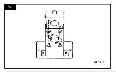
9.4 Feed the cable back through the hole as you replace the bracket. When the bracket is located correctly it will sit flush with the back panel without force being required. If not positioned correctly the bracket will sit at an angle (see Diagram 17).
