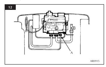
7.3 Reassemble the interrupter block and leads. Secure the thermocouple connection in the rear of the gas control. (Do not overtighten). Turn the gas supply on and check the entire pipe work and valve joints for any leaks.
