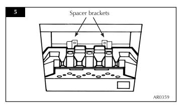
6.2 Locate the rear panel against the spacer brackets (see Diagram 3) and slide down so that it locates on the ledge of the flame baffle (see Diagram 6).
