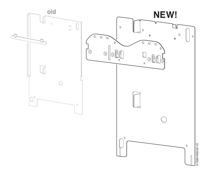
Due to continuous product improvement the mounting plate and the hanging bracket have been modified. Therefore some drawings in the installation manual of the appliance do not completely comply with the delivery. For the installation of mounting plate and hanging bracket refer to the back side of this sheet. All the other installation steps for the appliance keep untouched by this modification.
