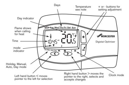
**NOTE:** The temperature displayed is actual room temperature unless adjusting the + or - button when the set temperature is displayed. Once adjustment is complete and after a 5 second delay the display will return to the actual room temperature.
