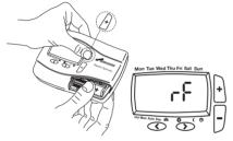
6. Remove the batteries from the transmitter and wait for the display to fade. Press and hold the '+' button while re-inserting the batteries and keep the button depressed until the display shows 'rF'. The transmitter is now in constant transmission mode enabling it to be correctly positioned within the home.
