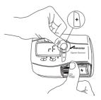
8. Press and hold the '+' button on the transmitter while re-inserting the batteries and keep the button depressed until the display shows 'rF'.
