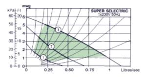
1. Set the speed selector switch to maximum (Speed 111) and switch on the electricity supply and start the heating system.
