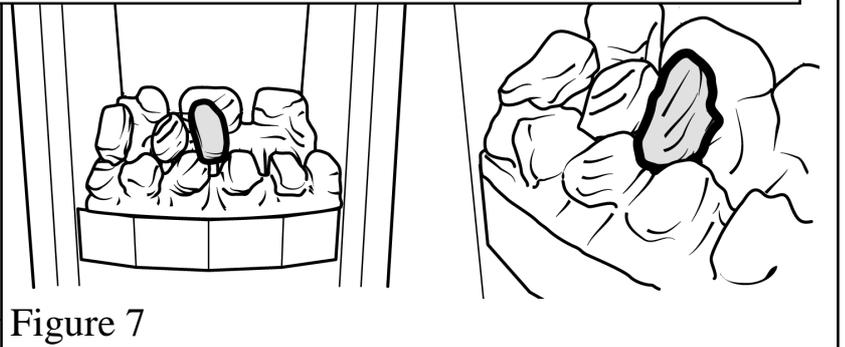
7. Place the remaining type "B" coal at the right side of the firebox between the front and rear base coals. Its two grooves should be on the top surface with the wide flat end to the front. The coal should touch the right side of the firebox. See figure 8.
