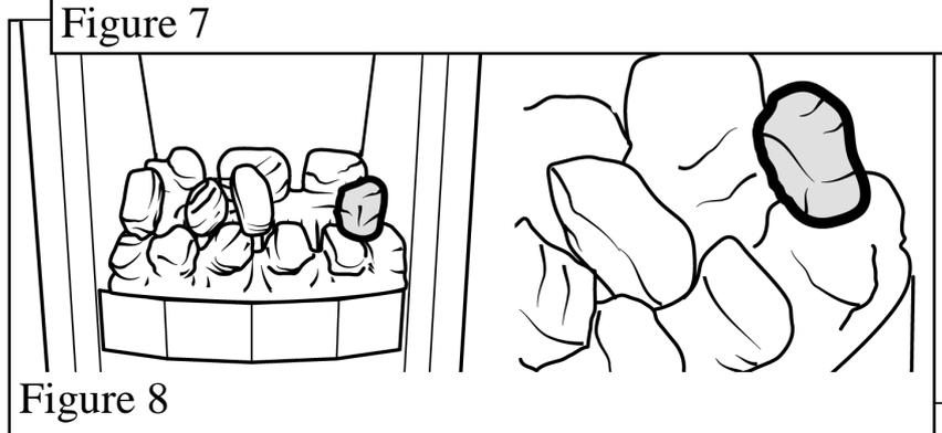
8. Place the remaining type "A" coal between the front and rear base coals with its lip to the front and its rear face between the right and centre coals of the rear base coal. Angle the coal so that the gap between it and the type "B" coal to its right is appreciably larger than the gap between it and the type "A" coal to its left but do not have it touching the type "A" coal. This will give the best flame effect. See figure 9.
