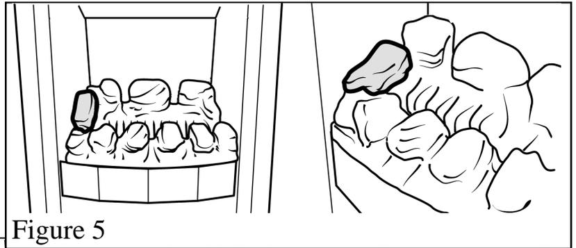
5. Place a type "B" coal between the front and rear base coals as shown in figure 6. Its two grooves should be on the top surface. Its wide flat end should be at the back between the left and centre coals of the rear base coal.
