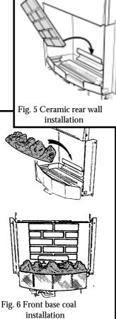
Install the 9 loose coals as follows. The smooth surfaces of the coals should be at the bottom and back.
