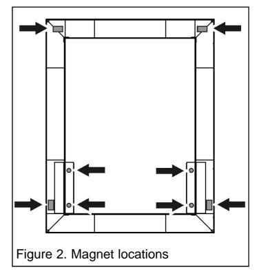
**3.** Keeping the lower part of the fascia away from the convection box flanges, offer the top of the fascia onto the support bracket (See figure 3). With this in place, swing the lower part of the fascia into place. The magnets will secure the fascia in place.
