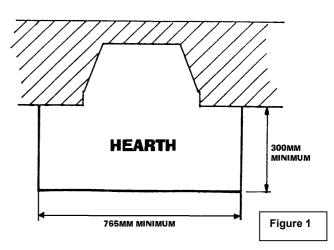
The surface of the hearth must be sufficiently flat to enable the bottom of the front surround and the bottom front cover to be aligned horizontally. Any excessive unevenness (uneven tiles, Cotswold stone, etc.) should be rectified. The appliance must not stand on combustible materials or carpets.
