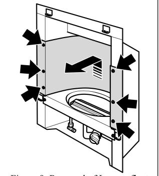
Figure 9. Removal of Inner reflector
