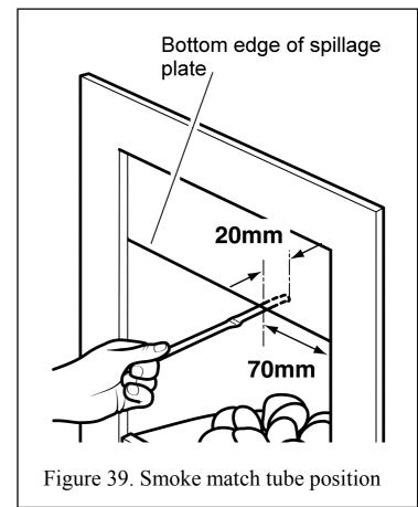
If the smoke is drawn into the appliance, continue with the installation. If the test is not satisfactory disconnect the appliance and advise the customer of the cause of failure.
