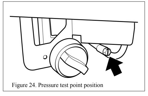
appliance alight and the control set at 'HIGH'. After checking the pressure, turn off the appliance. Remove the pressure gauge and replace the test point sealing screw. Re-light the appliance. Turn to 'HIGH' position and test around the sealing screw for gas soundness using a suitable leak detection fluid.
