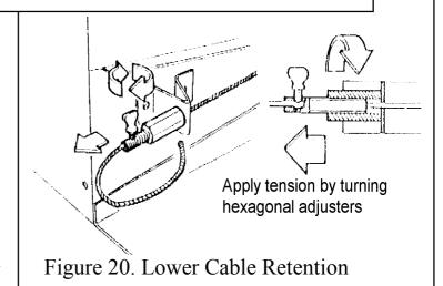
hotbox is aligned squarely and the sealing is satisfactory, fully tighten the cable retainers.
