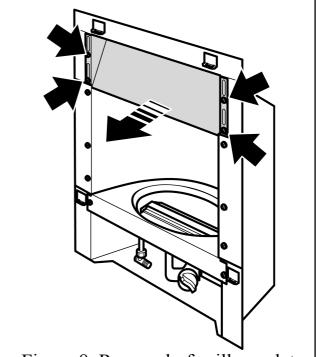
Figure 8. Removal of spillage plate
