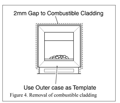
combustible cladding removal and that this area is increased by at least 2mm all round. If the cladding projects forward from the fixing plane of the fire the clearance at the top of the appliance must be increased to a minimum 15mm. This will allow for surround removal.
