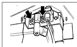
Figure 44. Pilot unit removal (Dust cage not shown for clarity)
