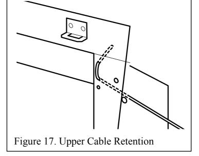
each upper side. Insert one end of each cable (one cable each side) from the back through the lower of the two holes and return the end through the upper of the holes. See figure 17. Give the cables a pull so that they grip against the hotbox flanges.
