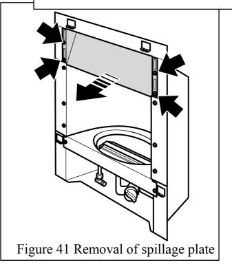
3. Detach the spillage plate from the hotbox by removing the four screws (See figure 41). Place the spillage plate in a safe place away from the work area.
