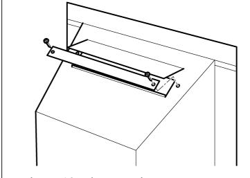
Figure 13. Flue Restrictor
