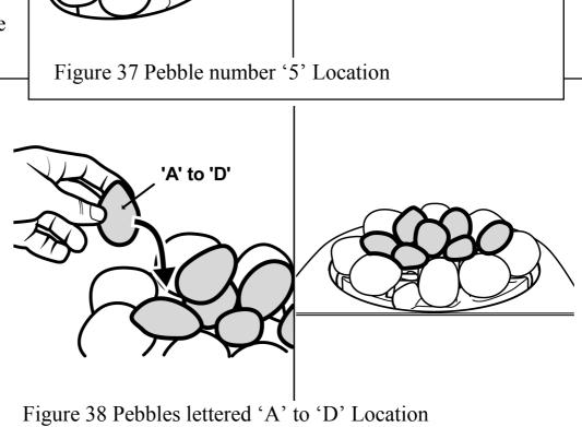
necessary to position these pebbles away from the centre of the fuel bed allowing more central flames.
