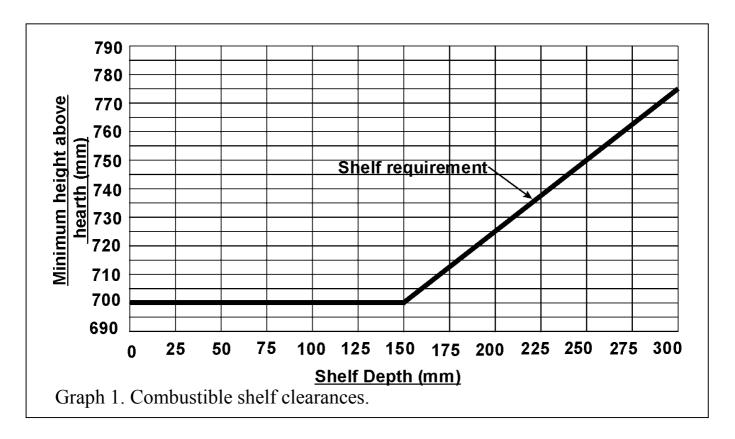
Combustible projections up to 75mm forward of the fixing plane of the fire to be a minimum of 125mm from the fireplace opening. Projections above 75mm forward of the fixing plane of the fire to be a minimum of 250mm from the fireplace opening. Non-combustible side projections to be 75mm from the fireplace opening
