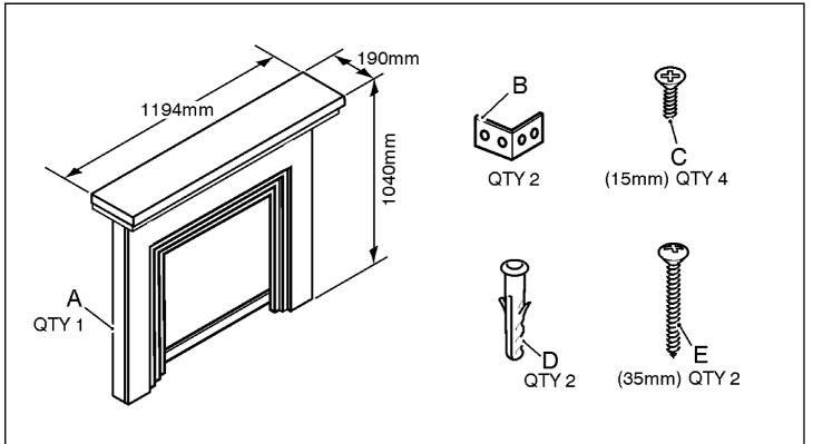
Figure 1. Contents (Items are not to scale. Any components extra to those above can be discarded).
