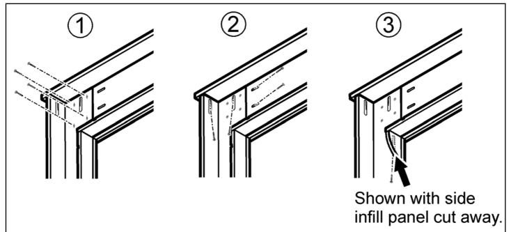
Figure 3. Securing the top to the legs (Repeat operations on both sides of the surround)
