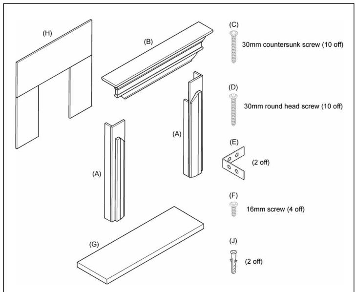
Figure 1. Contents - Fire not shown. (Items are not to scale. Any components extra to those above can be discarded).
