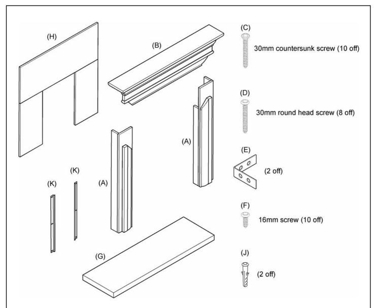
Figure 1. Contents - Heater not shown. (Items are not to scale. Any components extra to those above can be discarded).
