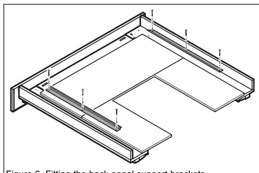
Figure 6. Fitting the back panel support brackets.
