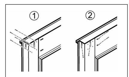
Figure 4. Securing the top to the legs (Repeat operations on both sides of the surround)
