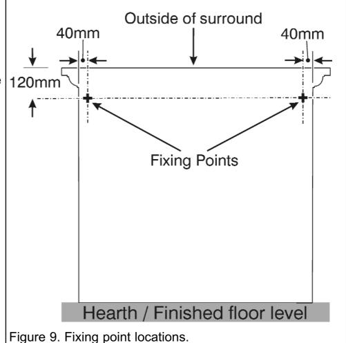
plaster board we recommend the use of heavy duty cavity fixings.
