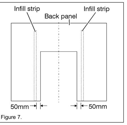
loosen the screws securing the strips to the brackets, adjust to the required depth and tighten the screws.
