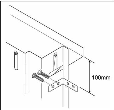
Figure 3. Fitting the wall brackets to the surround legs.
