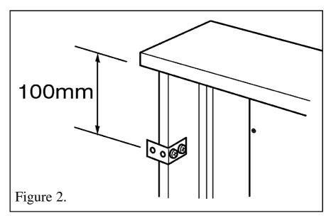
• Position the Surround and hearth set in place. Mark the positions of the bracket holes on the wall. Move the Surround and hearth set aside and drill suitable sized holes. Insert the wall plugs (D). Position the Surround and hearth set in place and secure using two screws (E).
