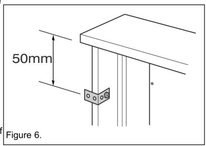
Position the assembly and secure using two screws (F).
