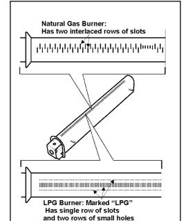
Figure 1 Burner Identification
