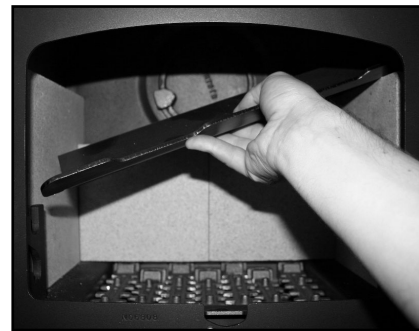
Fig. 6. Inserting Throat Plate in to the Valor Hamlet Multifuel.
