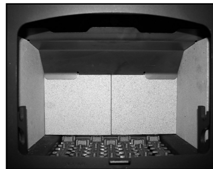
Fig. 7. Liners, throat plate and grate in the Valor Hamlet multifuel.
