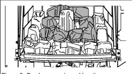
Figure 3. Overlay ceramic coal location
