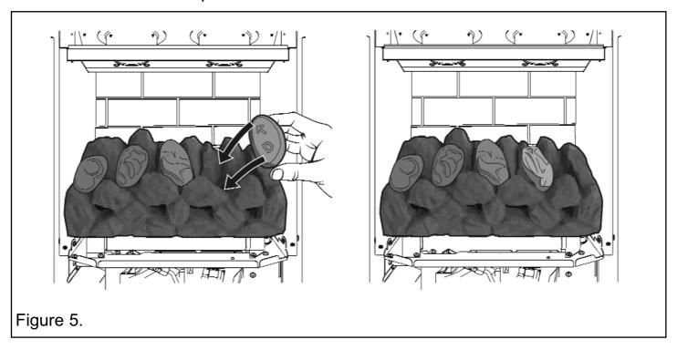
6. Locate ceramic coal 'E' onto the base ceramic as in figure 6. Ensure that the arrow on the underside of coal points to the rear of the fire.
