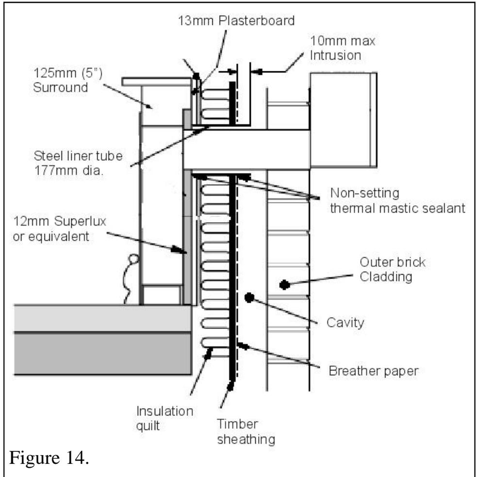
the usual 13mm plasterboard wall lining plus 12mm of “Superlux” or similar non-combustible material. The opening should be between studs.
