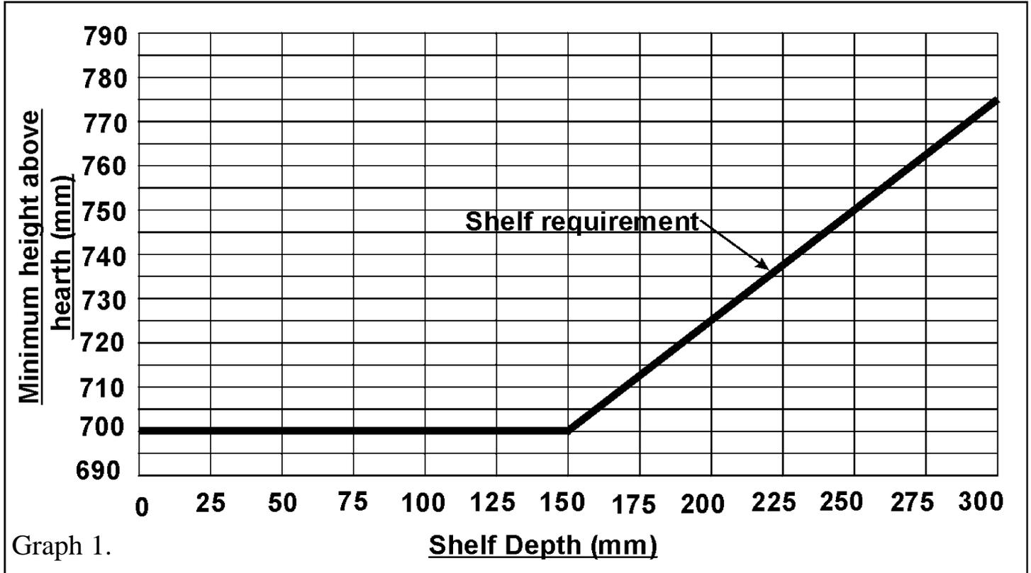
**3.1.9** The front face of the wall should be reasonably flat over the area that will be covered by the fire box top and side flanges to ensure a good seal. The minimum height from the top surface of the hearth to the underside of any shelf made from wood or other combustible materials is as follows:-
