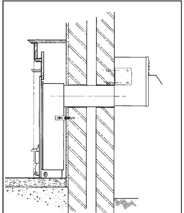
Figure 9. Main case in front of wall.
