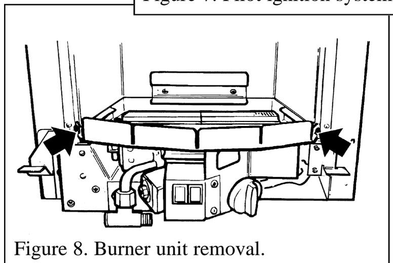
Figure 8. Burner unit removal.
