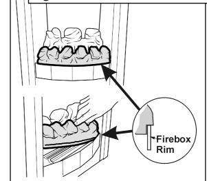
Figure 3 Front Base Coal Position
