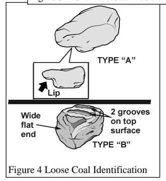
**4.** Place a type "A" coal between the front and rear base coals with its lip to the front and so that the coal is close to the left side of the firebox. See figure 5.
