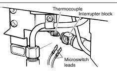
Fig. 43 Thermocouple Interrupter Block
