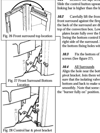
10.1 Remove the tape securing the control linking bar to the front surround. Slide the control button upwards as far as it will go. Make sure that the bottom of the linking bar is higher than the bottom of the front surround.
