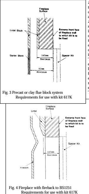
**2.3** With the addition of optional accessory spacing kit 617K together with a sufficiently deep surround and hearth, this appliance can be fitted in the following situations. Full installation requirements and instructions are provided with the kit.
