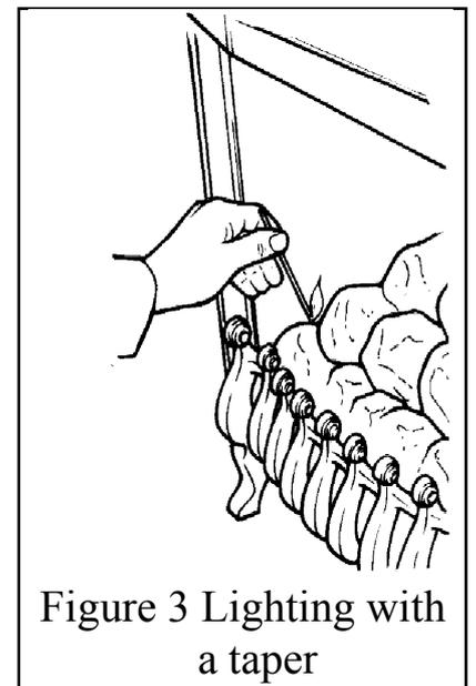
Figure 3 Lighting with a taper
