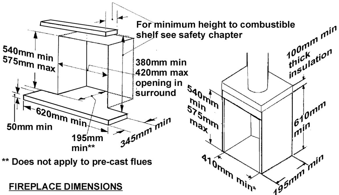
\*If internal width is greater than 440mm, the opening width must be reduced to not more than 440mm to ensure adequate sealing to the fire
