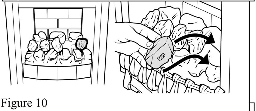
5. Place the remaining type "A" coal between the front and rear base coals. The letter "A" should be upside down with its rear face between the right and centre coals of the rear base coal. Angle the coal so that the gap between it and the type "B" coal to its right is appreciably larger than the gap between it and the type "A" coal to its left but do not have it touching the type "A" coal. This will give the best flame effect. See figure 11.
