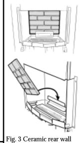
Fig. 3 Ceramic rear wall installation
