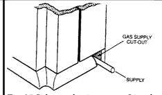
Fig. 25 Side supply pipe entry - Lincoln
