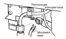
Fig 43 Thermocouple interrupter block
