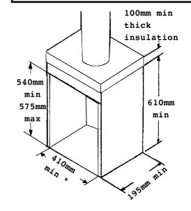
\* If internal width is greater than 440mm the opening width must be reduced to not more than 440mm to ensure adequate sealing to fire.
