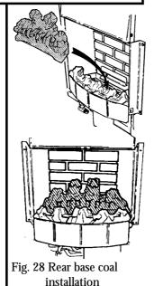
10.4 Install the 9 loose coals as follows. The smooth surfaces of the coals should be at the bottom and back.
