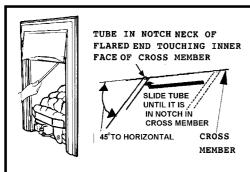
Fig. 34 Smoke match tube position (Monaco front shown)
