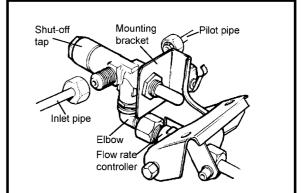
Fig. 45 Shut-off tap (viewed from rear with burner turned over)
