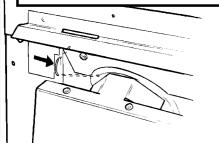
Fig. 17 Upper cable retaining
