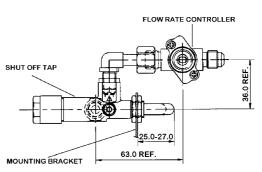
Fig. 46 Refitting dimensions of valves into mounting bracket
