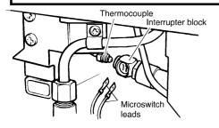
Fig. 37 Thermocouple interrupter block
