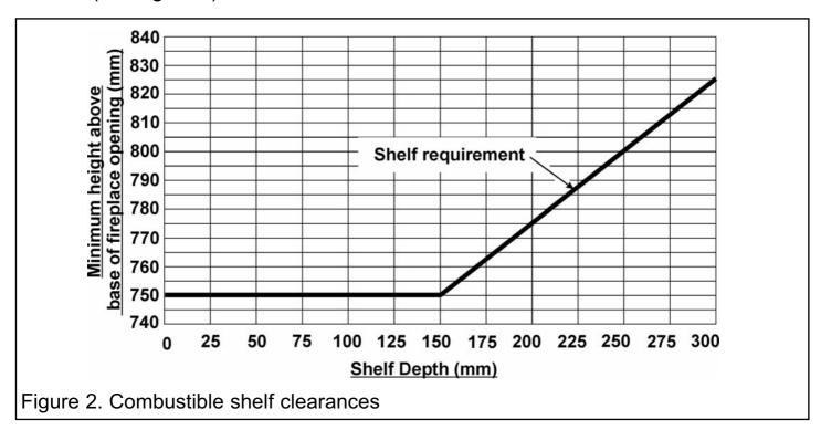
**3.9.2** The minimum allowable distance from the outside of the fascia to a corner wall having combustible material or any other combustible surface which projects beyond the front of the appliance is 100mm.
