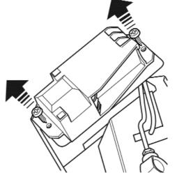
Figure 29. Removal of electronic spark generator
