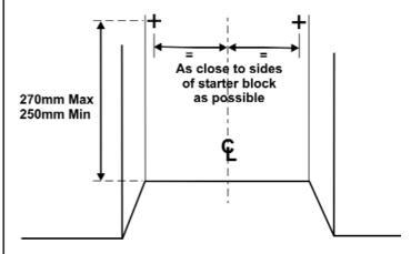
For pre-cast flue installations where the width of the opening / pre-cast starter block is less than 300mm.
