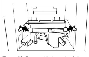
Figure 28. Burner attachment points
