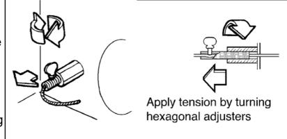
itself. Pull each cable taut again and push the cable retainers back against the back panel. Again, tighten the screws in the retainers and apply tension to the cables by
