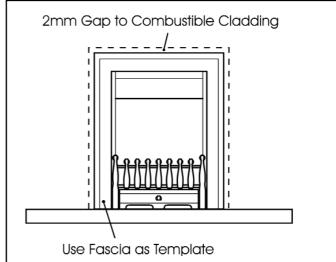
Figure 1. Removal of combustible cladding (Fascia may differ from that shown)
