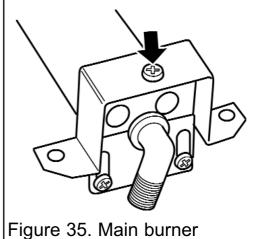
Figure 35. Main burner Injector removal
