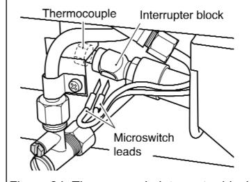
Figure 24. Thermocouple interrupter block
