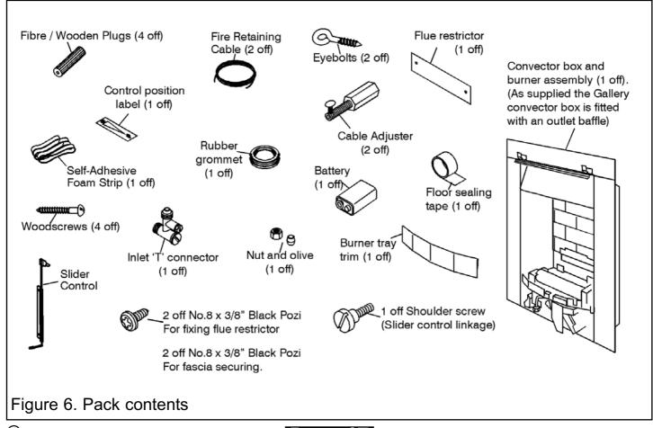
Remove all the items carefully to prevent damage. Take special care when handling the ceramic components. Some items may be contained in the packaging fitments - Examine the packaging carefully before discarding. Check that all the items are present and undamaged.
