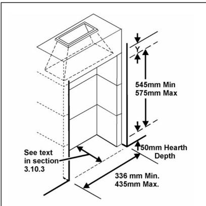
Dimension 'Y' to be made up with suitable noncombustible building material.
