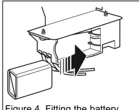
Figure 4. Fitting the battery
