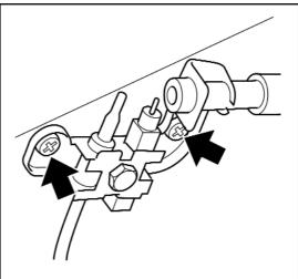
Figure 31. Pilot unit removal
