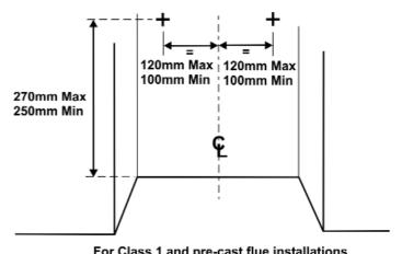
For Class 1 and pre-cast flue installations where the width of the opening / pre-cast starter block is 300mm or greater.
