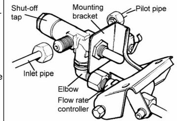
Figure 32. Shut-off tap (Viewed from rear with burner turned over)
