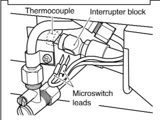
Figure 30. Thermocouple interrupter block
