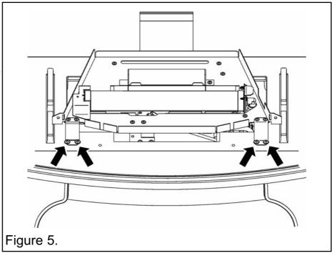
body of the stove is not shown for clarity). The rear leg of the burner should sit in the recess at the rear of the casting and on top of the two lugs that protrude. Secure using the screws supplied.
