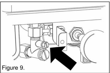
• Relight the appliance. Turn to the maximum output position and test around the sealing screw for gas soundness with a suitable leak detection fluid.
