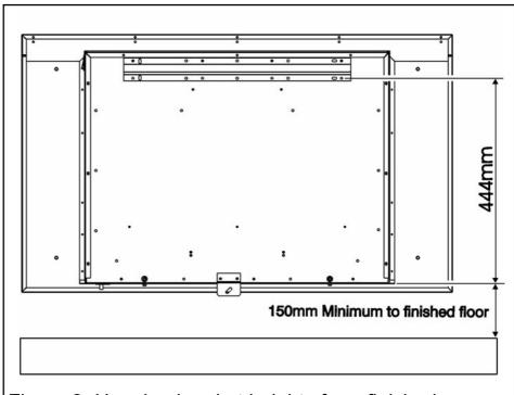
Figure 3. Hanging bracket heights from finished floor / hearth
