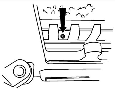
Figure 6. Removing the black metal basket
