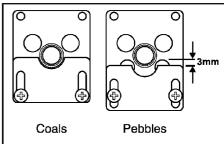
Figure 29. Aeration shutter settings for 'coal' and 'pebble' ceramic fuel effects.
