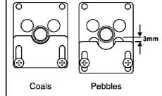
Figure 29. Aeration shutter settings for 'coal' and 'pebble' ceramic fuel effects.
