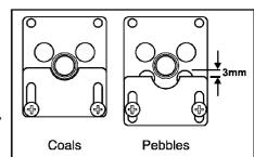
Figure 29. Aeration shutter settings for 'coal' and 'pebble' ceramic fuel effects.
