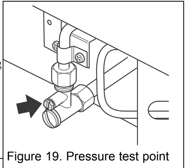
Figure 19. Pressure test point
