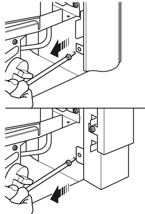
Figure 48. Removing the surround fixing screws
