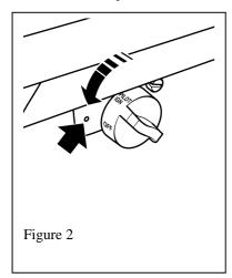
When the burner is alight at its low setting, partially depress the knob and gradually turn it anticlockwise until the burner is at your desired level. The burner flames will gradually increase until the knob reaches the "HIGH" position.
