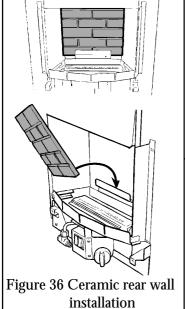
12.1 With its feather edge at the top, place the ceramic rear wall into the channel at the back of the fire box. Push the wall flat against the rear of the fire box. (See figure 36) .
