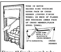
Figure 43 Smoke match tube position
