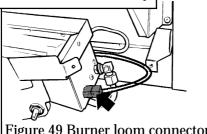
Figure 49 Burner loom connector
