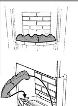
12.2 Place the two halves of the front base coal in the burner compartment so that they rest on the ledges at the sides and front. Pull the coals forward so that they are immediately behind the front rim of the burner compartment (See figure 37).
