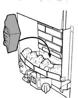
Figure 38 Rear base coal installation
