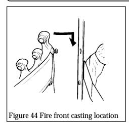
14.1 All models except black & chrome front casting. Fit the fire front casting to the front surround. Locate the two screw heads at the rear top corners of the casting through the keyhole slots at the inner sides of the surround. If the screw heads do not project enough or project too far, the screws can be adjusted. Lower the casting so that it rests on the hearth (see figure 44).
