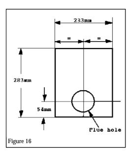
**6.12** Drill the flue hole through the wall. The hole centre should be on the flue duct centre line. For buildings constructed of brick, stone etc use a  $3\frac{1}{2}$  in. (89mm) core drill.
