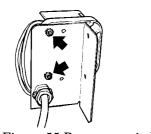
Figure 55 Pressure switch fixings
