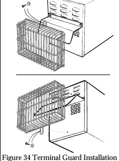
Fit the weather shield and guard to the back of the flue unit as detailed below (see figures 33 & 34).
