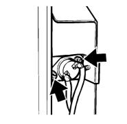
Fig. 21 Flue Switch Screws
