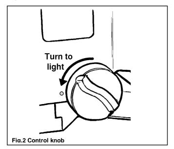
Depress the control knob and turn anticlockwise towards the PILOT/IGN position (Figure 2). A spark should be generated at the pilot while turning. The spark should ignite the pilot. The pilot flame can be seen below round coal at the front left side.
