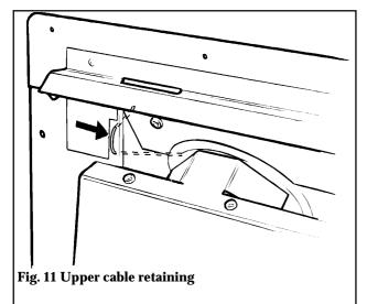
**7.2.5** Thread the cables through the upper eyebolts in the rear wall and then through the lower eyebolts. Return the cables through the holes near the bottom of the convection box back panel and through the "V" shaped brackets near the bottom front sides of the convection box (see figure 12).
