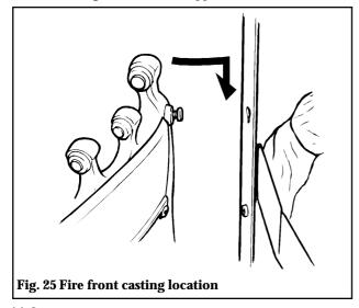
**11.2** Place the bottom front cover casting in position below the fire front casting.
