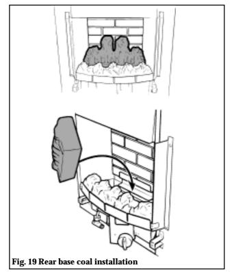
**9.4** The ceramic side walls are marked at the rear bottom corners "L" (Left side) & "R" (Right side). Place the side walls against the sides of the fire box and in the recesses at the sides of the base coals. The markings "L" & "R" should be at the at the back bottom corners and facing to the centre of the back of the firebox (See figure 20).
