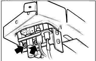
Fig. 29 Pilot unit attachment points (Dust cage not shown for clarity)
