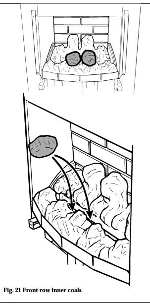
**9.5.2** Place two of the remaining coals in the two outer valleys of the front coal (One each side of the large coals) (See figure 22). Place the left side coal so that the customer will be able to see the pilot flame below the coal.
