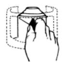
TO TURN THE GAS ON continue turning the switch clockwise so that it points UPWARDS to the FLAME SYMBOL. The valve is now open and the gas is ON. Light the heater. Follow the lighting instructions on the heater cabinet.
