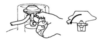
TO TURN THE GAS OFF turn the switch anti-clockwise to the LEFT. DO NOT TOUCH THE CENTRE BUTTON.
