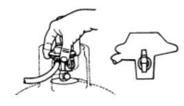
ENSURE that the point on the switch is pointing DOWN. Place the regulator down over the cylinder valve.
