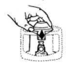
TURN the black switch anti-clockwise so that it points to the LEFT (the OFF position – Fig 2a). CHECK THAT THE HEATER AND PILOT ARE OUT. Remove the cylinder from the heater then, and only then, should the switch be turned anti-clockwise to the DISCONNECT position (DOWNWARDS).
