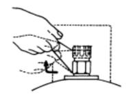
PULL the lanyard out then upwards. The cap will lift off the valve. Do not use tools. Leave the cap hanging down from the valve while the cylinder is in use.
