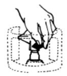
**c** FIT the regulator/adaptor on to the cylinder valve and turn the black switch clockwise so that it points to the LEFT ( the OFF position). The regulator/adaptor is now secured gas tight to the valve which is still closed-OFF. Place the cylinder in the heater.
