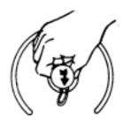
**a**ROTATE the plastic cap on the CYLINDER VALVE until the arrow points out through the gap in the valve shroud.
