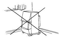
DO NOT position the heater alongside a wall or near curtains etc. ALWAYS face the heater towards the centre of the room. Special care should be taken if the heater is on a surface where it can move or twist on its wheels or castors if knocked by a child or dog etc.
