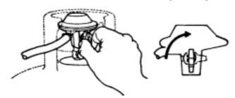
TO TURN THE GAS ON turn the switch clockwise so that it points upwards. The cylinder valve is now open and the gas is ON.
