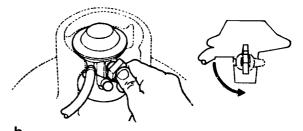
KEEPING the button in the depressed position, turn the black switch anti-clockwise until it points downwards. The regulator can then be lifted off the valve.
