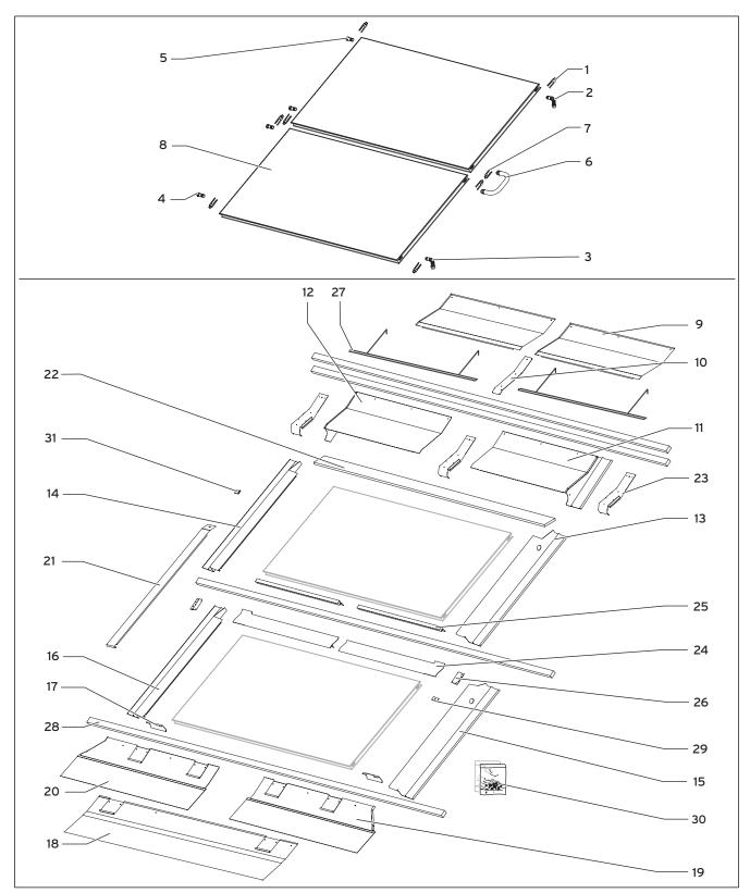
Fig. 4.2 Horizontal collector mounting kit
