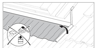
· Bend the flexible protections on the collector field ends.
