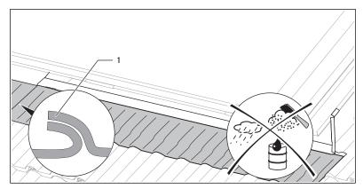
Fig. 4.39 Adapting the flexible protection
