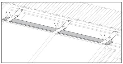
Fig. 4.33 Mounting the support boards
