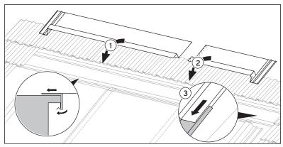
Fig. 4.29 Mounting the ridge plates (roof angle 15-22°)
