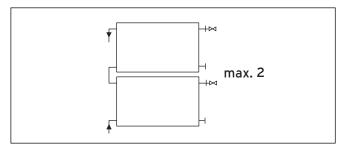
Fig. 4.5 Field arrangement on top of each other
