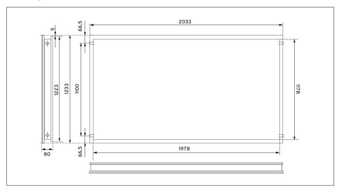
Fig. 7.1 Scale drawing VFK 145 H, VFK 150 H
