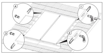
Fig. 4.25 Mounting the hydraulic connections (1-5 collectors)
