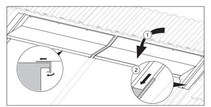
Fig. 4.34 Mounting the ridge plates
