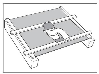
Fig. 4.8 Feeding the pipe through the sarking membrane
