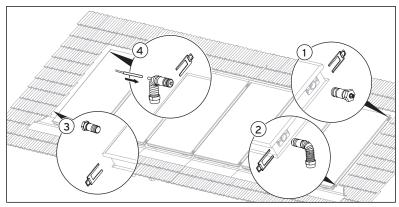
Fig. 4.26 Mounting the hydraulic connections (6-12 collectors)
