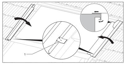
Fig. 4.22 Fixing the upper side sections
