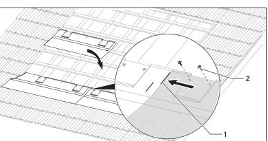
supplied Torx bit screw it to the roof batten with the 6 supplied sealing bolts (bolts • Gradually fix the remaining frame compo-
