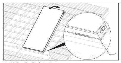
Fig. 4.13 Inserting the right collector
