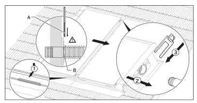
Fig. 4.24 Inserting the remaining collectors
