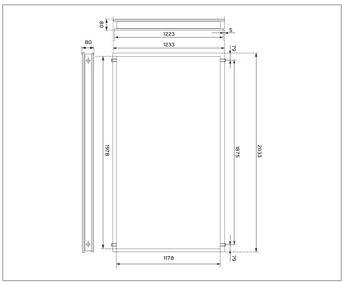
Fig. 7.3 Scale drawing VFK 145 V, VFK 150 V  $\,$
