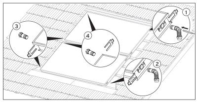
Fig. 4.19 Hydraulic connections
