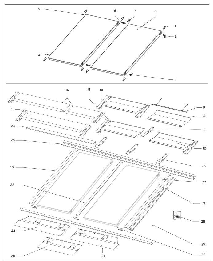
Fig. 4.1 Vertical collector mounting kit
