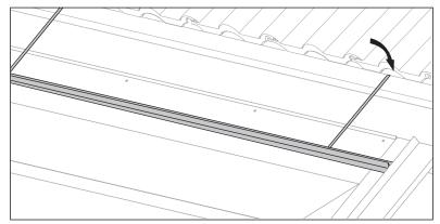
Fig. 4.37 Covering the profile ends
