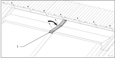
Fig. 4.35 Ridge plate coupling
