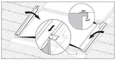
Fig. 4.20 Fixing the lower side sections
