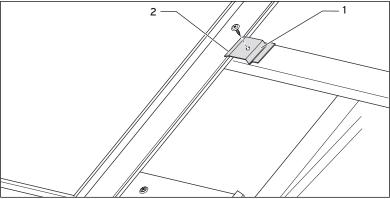
Fig. 4.14 Screwing the flat collectors
