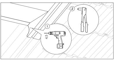
Fig. 4.36 Rivetting the frame
