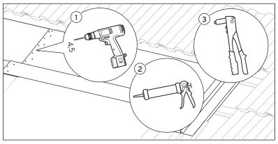
Fig. 4.30 Joining the ridge plates (roof angle 15-22°)
