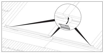
Fig. 4.38 Covering the profile ends
