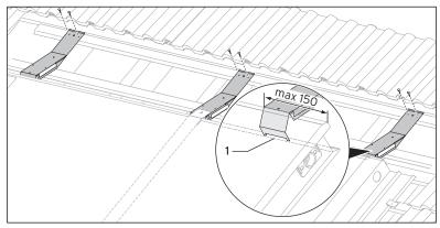
Fig. 4.32 Mounting the support plates (vertical collector)
