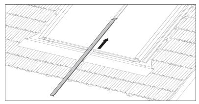
Fig. 4.28 Attaching the vertical intermediate plate
