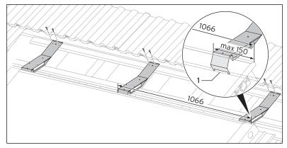
Fig. 4.31 Mounting the support plates (horizontal collector)
