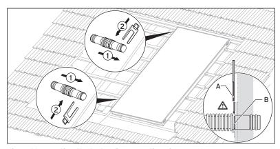
Fig. 4.23 Mounting the hydraulic connection pipes
