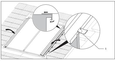
Fig. 4.27 Screwing the side sections
