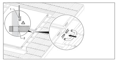
Fig. 4.18 Hydraulic connection
