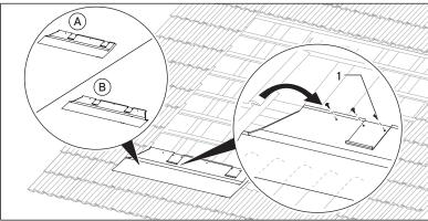
Fig. 4.11 Mounting the left lower frame
