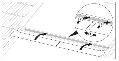
Fig. 4.21 Fixing the horizontal intermediate plates
