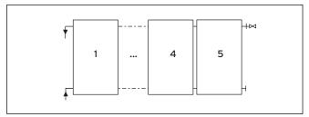
Fig. 4.3 Field arrangement side by side for 1 - 5 collectors
