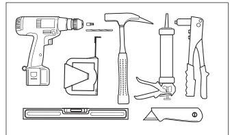
Fig. 4.9 Installation tools: water level, cordless screwdriver,
