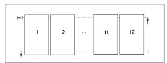
Fig. 4.4 Field arrangement side by side for 6 - 12 collectors
