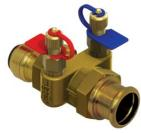
DZR metering station. DZR brass body with test points, XPress press end x Tectite push end for copper/carbon steel/stainless steel tube.
