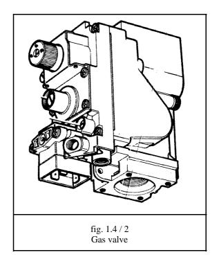
All the setting and regulation operations have to be made by professional qualified people. In case of valve replacement, be sure that the gas flow is in the direction of the arrow on the body the valve and while installing care should be taken to ensure no foreign matter enters into the valve. MAINTENANCE: the only operation allowed is the solenoid replacement, which has to be carried out by qualified personnel..
