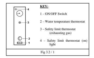
To check the operating of the thermostat, turn the knob 2 (pict. 3.2/1) to the lower value and check that the burner extinguishes. Turn the knob again to the previous pre-set value and check for a proper ignition of the burner.
