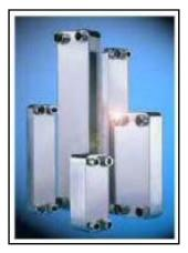
With a maximum flow rate of up to 200 m<sup>3</sup>/Hour, most duties will be covered. The majority of our brazed heat exchangers are a stock item. The standard unit is manufactured from stainless steel grade AISI 316 and is brazed with pure copper. Although these units are classed as standard, there is a large range of units with different connection sizes and orientations etc, which ensures we can supply a unit for your requirements.
