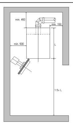
Diagram showing clearances required in boiler room.
