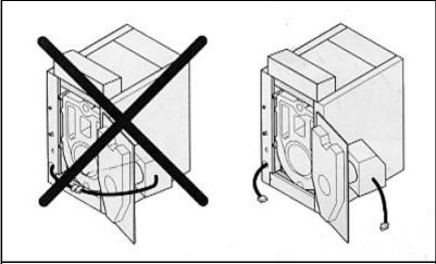
When connecting the burner, make sure the length of the burner cable is such that when the burner door is opened it becomes disconnected.
