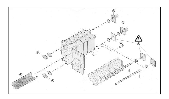
The order of assembly from (1) to (13) must be observed.
