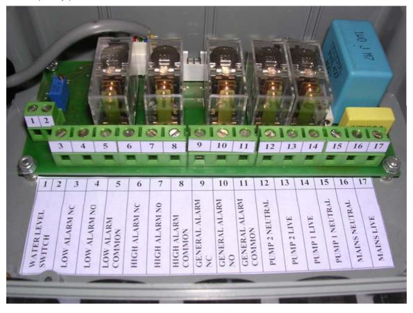
Connectors 1 and 2 are for the water level sensor and can be wired either way. The electronics use a 24V DC current for this purpose.
