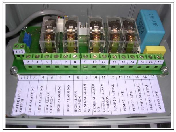
Connectors 1 and 2 are for the water level sensor and can be wired either way. The electronics use a 24V DC current for this purpose. If this option is not required then a loop of wire across these terminals is required. Please note however that the wires going to and from the level sensor must be protected in accordance to local regulations.
